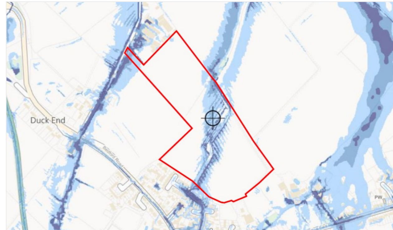
EA Flood Map for Planning extract, showing the pluvial (surface water) flood risk for the site.
