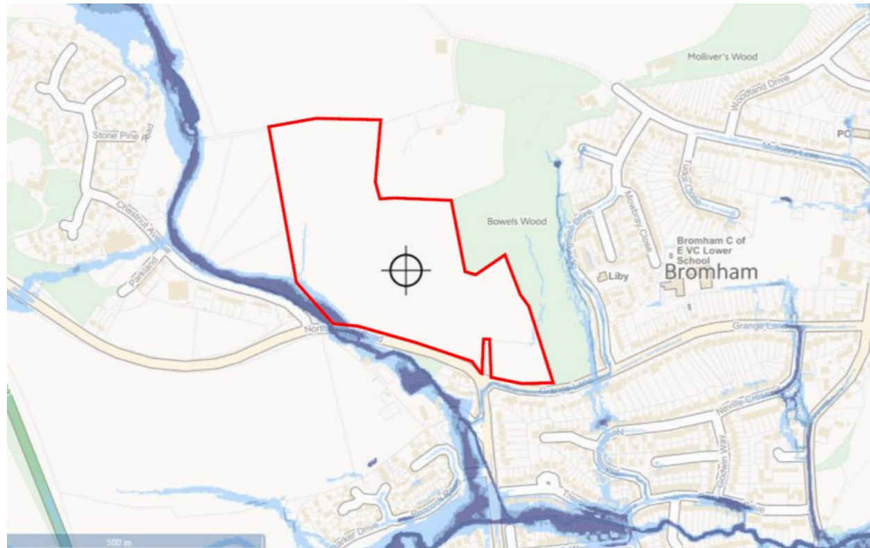
EA Flood Map for Planning extract, showing the pluvial (surface water) flood risk for the site
